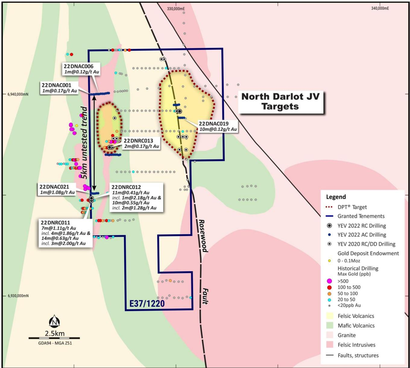
Figure 2: North Darlot project local geology and drilling
