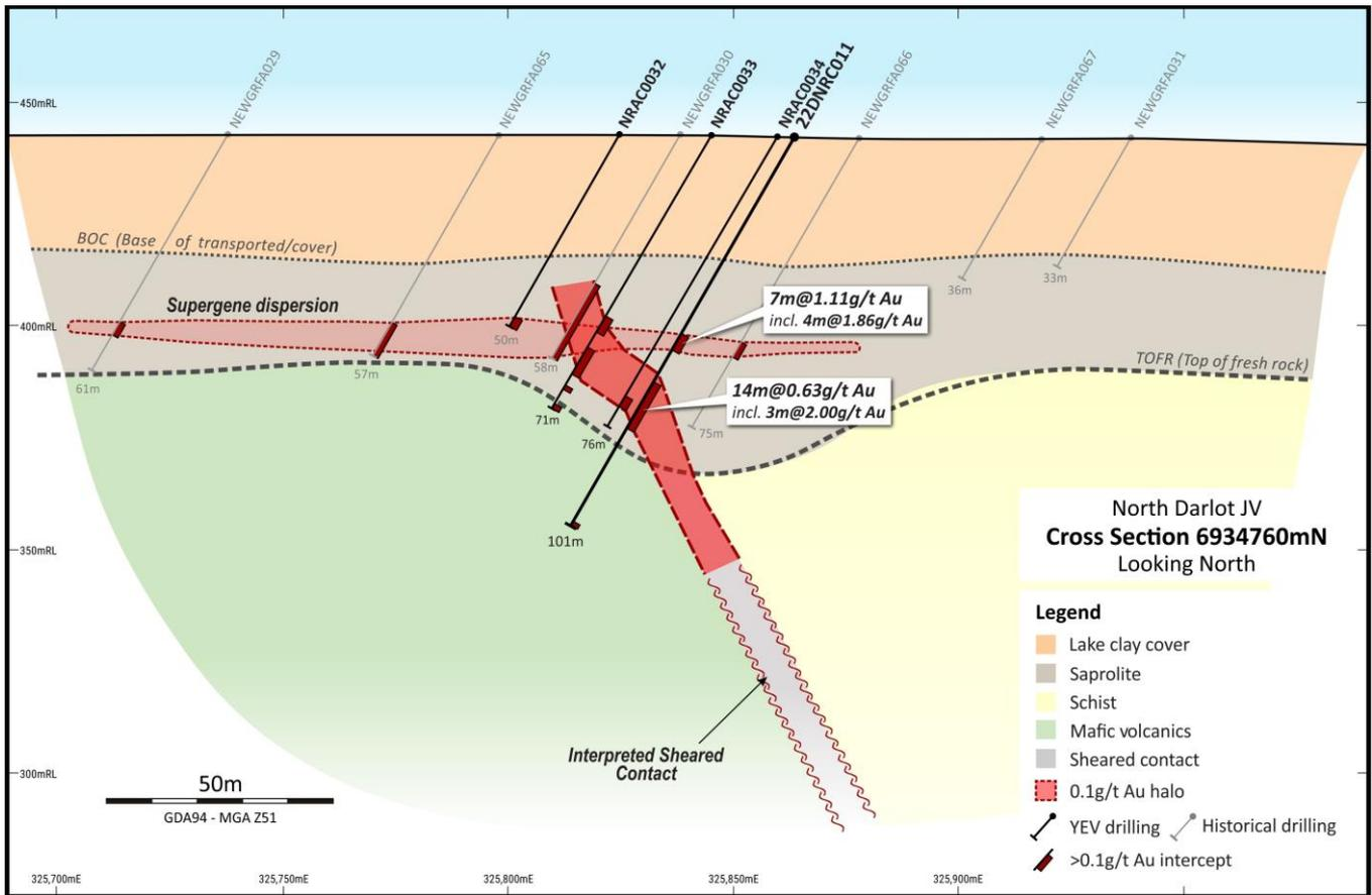
Figure 3: North Darlot project cross section 6934760mN looking north
