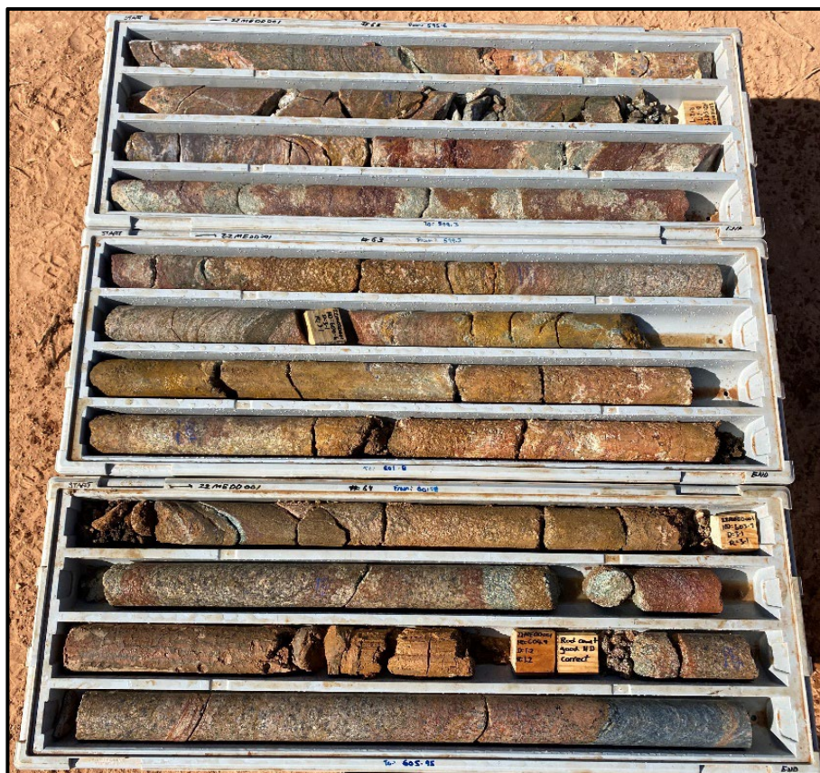
Figure 6. 22MEDD001, 595-605m, oxidised weathered low angled fault zone.
