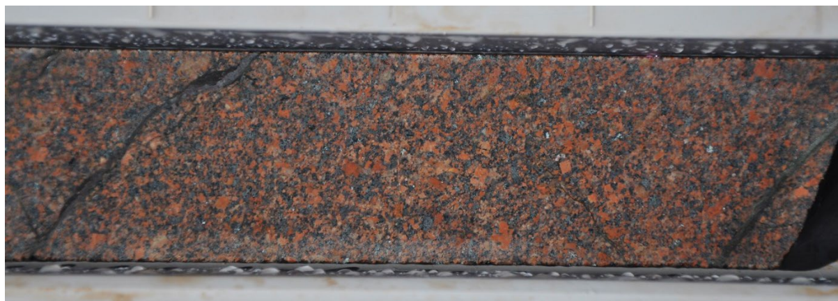
Figure 3: 22MEDD001 magnetite, hematite, albite, sericite, chlorite and epidote alteration in monzodiorite at 702m
