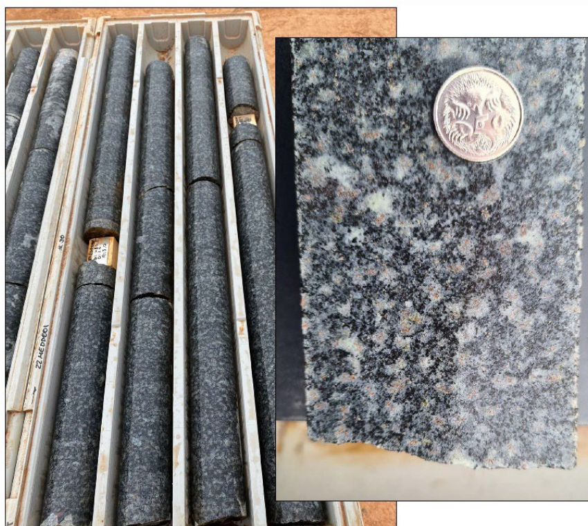
Figure 7. 22MEDD001, 509m. Biotite-hornblende-magnetite quartz monzodiorite with magnetite, 3% titanite, and minor apatite.
