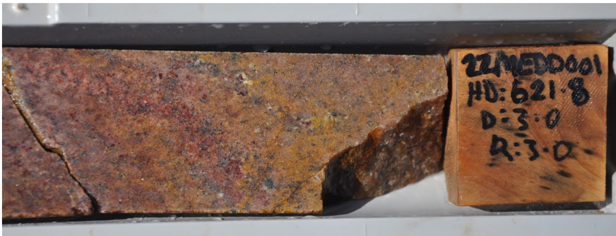
Figure 2: 22MEDD001 hematite, albite, sericite, chlorite, epidote, and pyrite alteration in syenogranite at 621.6m
